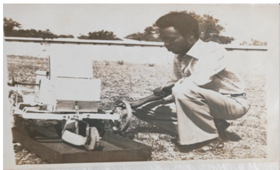
Figure 2: Calibrating planter/fertilizer applicator metering units
